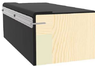
Installation on a wooden upstand
