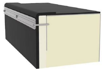
Installation on a steel sheet frame
