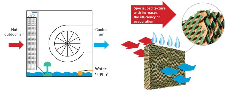
FES evaporative cooling units draw hot air through wet pads by using blower. As water evaporates from the pads it takes heat from the air with it, resulting in cooled air
