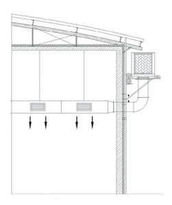
**Bottom-Blowing Installation**FESKLİMA 35RCB - 20RPB - 16RPB - 10RPB - 30APB - 25APB
