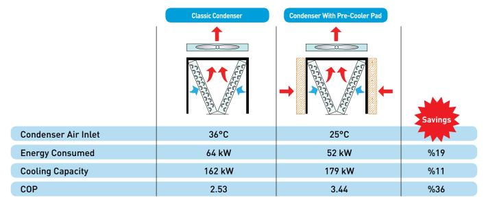
The savings are illustrated on the table above for Air cooled condensers with and without FESChill unit. As a result of 11°C decrease in inlet air, the energy consumed by the Chiller is decreased by 19% and the cooling capacity is increased by 11%. This allows the EER or COP of the chiller to increase by 36%. On average every 1.8°C decrease of air inlet temperature achieved by the pre-cooling pads, increases the condenser effectiveness by 2 %.
