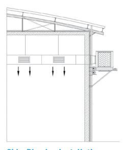
**Side-Blowing Installation** FESKLIMA 35RCS - 20RPS - 16RPS - 10RPS
