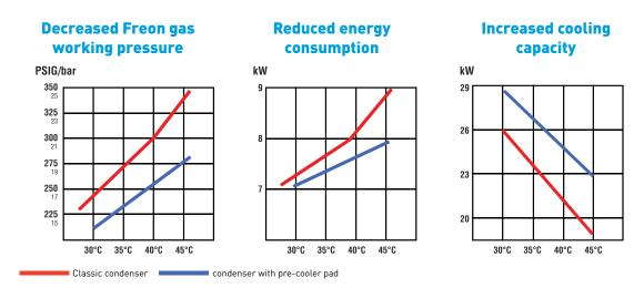
The condenser's air inlet decreases the system's working pressure, which creates increased cooling capacity and decreased energy usage.
