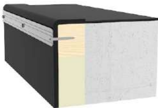
Assembly on concrete edging
